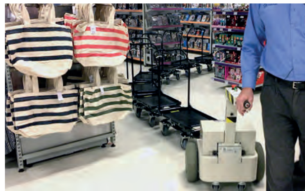
Follow-Me Trolleys in a train easily negotiating an S-bend.
